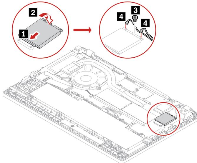
**Note:** When you install the wireless WAN card, ensure that you connect the orange cable to the main connector on the card, and the blue cable to the auxiliary connector on the card.
